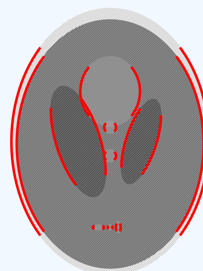
Visible singularities of Head-Phantom Angular range \Theta = [45^\circ, 135^\circ]
