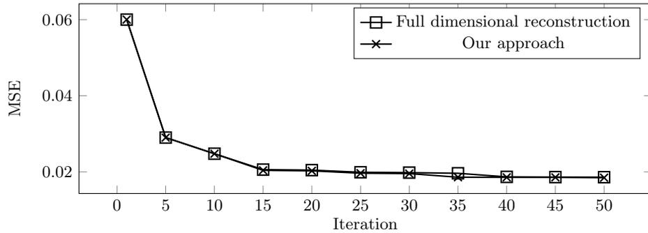
Figure 1: Tomographic reconstruction from limited angular range  $1^\circ \leq \theta \leq 90^\circ$ ,  $\Delta\theta = 1^\circ$ , using  $\ell^1$ -norm regularization of curvelet coefficients. The image quality obtained after dimensionality reduction (c) is as good as in the case of full dimensional reconstruction (b). However, the computational time for 50 iterations was significantly lower using our approach.
