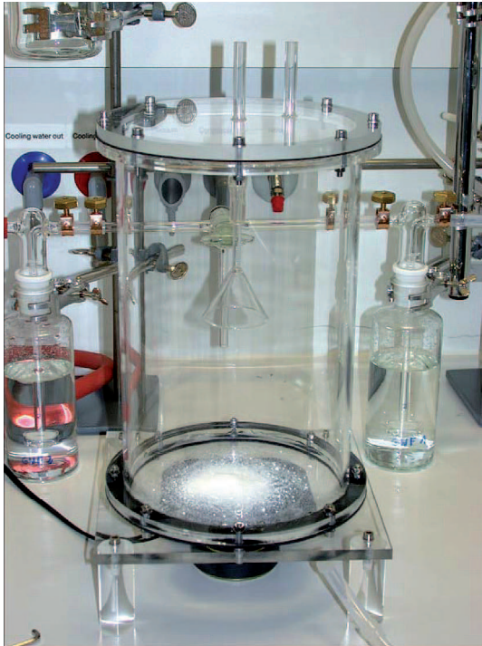
Figure 2: Set-up of the air-to-water transfer device with two washing flasks (background). In the foreground a NP-cloud generator where \text{TiO}_2 -NPs (white powder on bottom) are catapulted into the air by vibrations of a loudspeaker.
